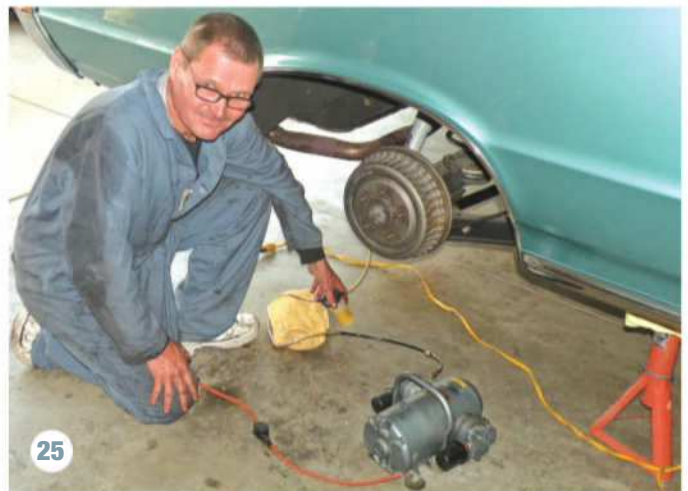
25 My buddy and chief mechanic brought his electric vacuum pump for the final bleeding. After a few tries, we removed all the air bubbles from the system, refilled the master cylinder, put the wheels back on, and went for a ride.
