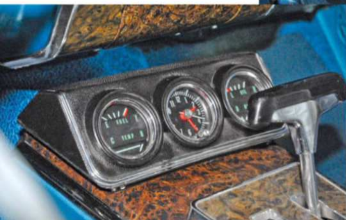
Interior looks original but boasts leather upholstery, Camaro console gauges, aftermarket wood-rim steering wheel, and CD changer. Cruise control and overdrive transmission are also concealed upgrades.
