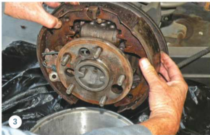
3 After giving everything a good spraying with aerosol brake cleaner from the local auto parts house (for a job like this, you'll probably need a few cans), the brakes were disassembled. Having a pot or other receptacle under the work area will keep your garage floor free of contaminants.
