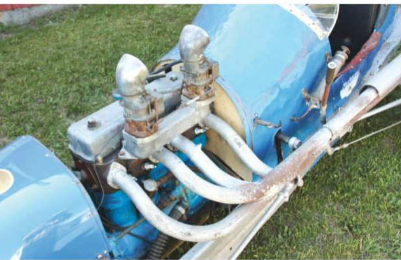
The pushrod overhead-valve Alexander (left) uses dual Stromberg 97 down-draft carburetors, a hot-rod favorite. The dual overhead-cam HAL breathes through side-draft Winfields, the period racing carb of choice. Both cars use magneto ignition, push start.
