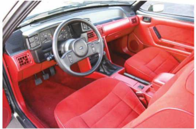
For 1987, the LX got cloth low-back seats as standard. The dash, console, and steering wheel were all newly restyled for that year.
