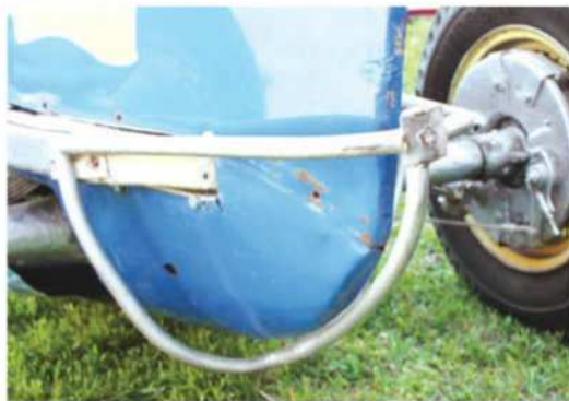
Nerf bar on the Alexander serves as "starter" allowing pushes from behind; previous practice was to tow start. Extra-deep bellhousing mates Model A transmission to Model B engine.
