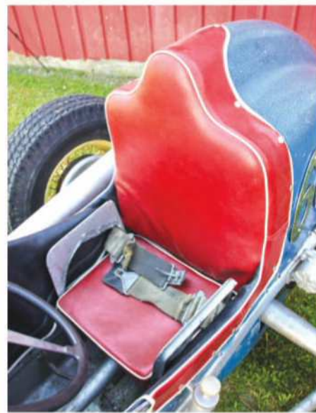
Restoration was generally avoided except where needed, such as replacing decayed original upholstery with new material. HAL features Dayton wheels – pricier than OE wheels on Alexander.
