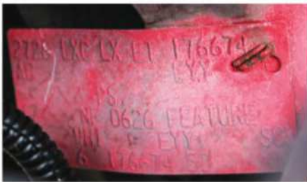
Fox Mustangs received metal tags fastened to the radiator support that listed equipment and trim codes.
