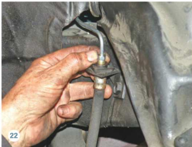
22 Once the front line is in position, it is connected to the front rubber flex hose. You may find it easier to pull the clip fastening the hose so that it can be moved to mate with the threaded fitting of the new line. But, don't fully tighten the fitting until the hose is re-fastened in its bracket.
