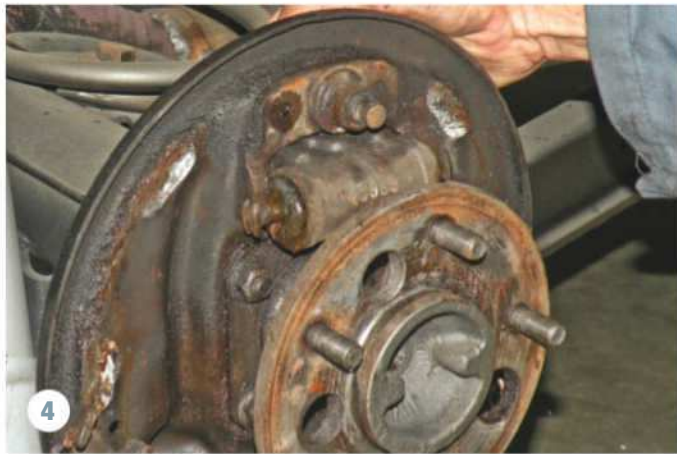
4 You can change a wheel cylinder without completely disassembling the shoes and springs, but we wanted to clean everything, including the backing plate, and it is a bit easier to get the cylinder out this way. The cylinder bolts and brake line attach to the cylinder from the rear of the backing plate. A movable light is handy for this task.
