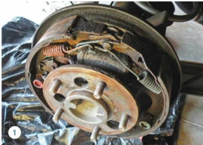
1 We began by jacking the car up and placing it on four sturdy jack stands before removing the wheels and then pulling the rear drums to inspect the rear wheel cylinders, as we suspected the trouble was in the rear. As soon as the drum was off, we could see that this wheel cylinder had definitely been leaking for a while.
