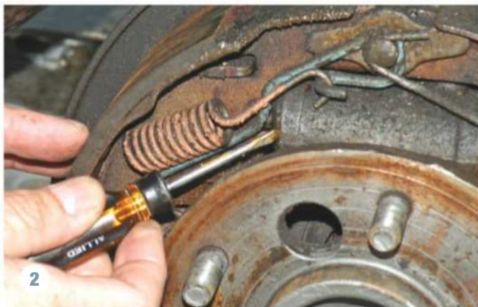
2 We checked the rubber seals on both sides of this wheel's cylinder and they were total junk. They had been leaking slowly for some time, obviously since before the obstruction in the main line. This wheel cylinder and the surrounding parts will all have to be removed and thoroughly cleaned. Brake fluid also destroys paint, so be careful taking these pieces apart.
