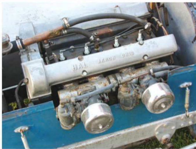
The pushrod overhead-valve Alexander (left) uses dual Stromberg 97 down-draft carburetors, a hot-rod favorite. The dual overhead-cam HAL breathes through side-draft Winfields, the period racing carb of choice. Both cars use magneto ignition, push start.
