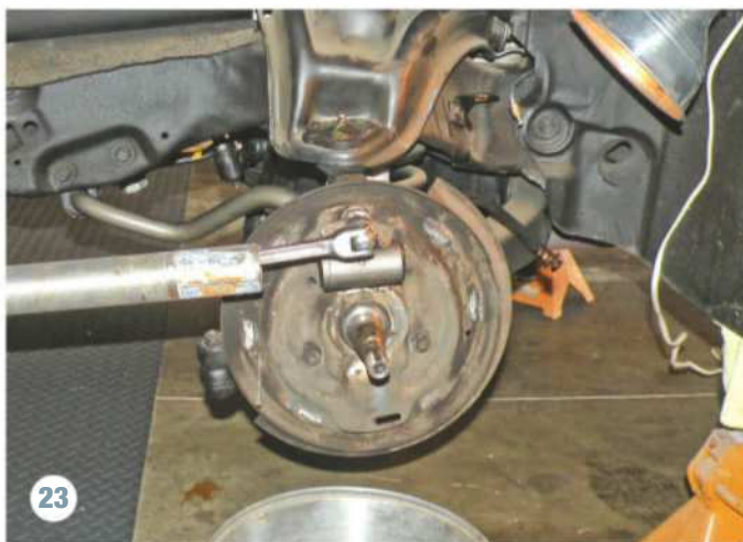
23 The new front-wheel cylinders have been installed, and here the front brakes are being reassembled. Again, white grease is used on the backing plate's shoe contact points to ensure smooth operation.
