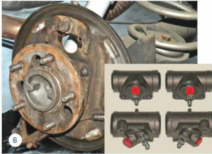
6 This corner is now ready to receive the new cylinder and cleaned-up brake parts. We purchased a full set of new wheel cylinders—notice that the fronts and rears are not the same. The areas that have the white patches are the pads where the brake shoes make contact—these should be sanded smooth if rusty, and then coated with some white grease.
