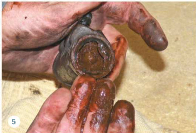
5 This is the mess we found at the passenger-side cylinder. Funk and rusty fluid was everywhere. If you attempt this work, take time to immediately wash the brake fluid from your hands – it's nasty stuff.
