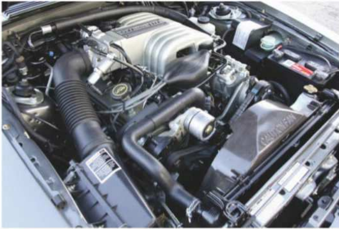
Ford's 5.0L HO V-8 received EFI for 1986; for 1987 output increased to 225 hp. This '88 has MAP engine management, with no mass-air meter.
