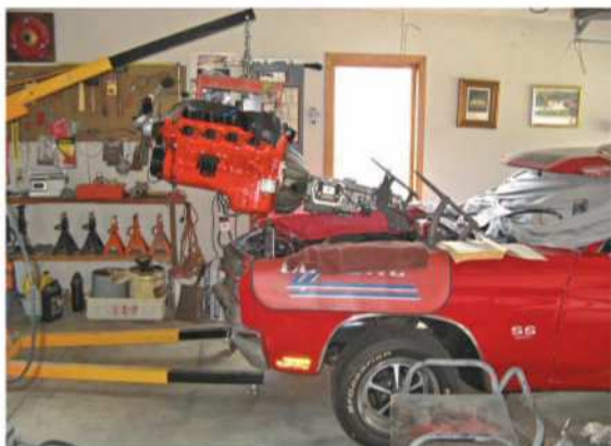
This Chevelle came with a rebuilt (but non-matching) 396 that proved to be sound once the restoration was first completed. Later, Donald built a 454 to take its place.
