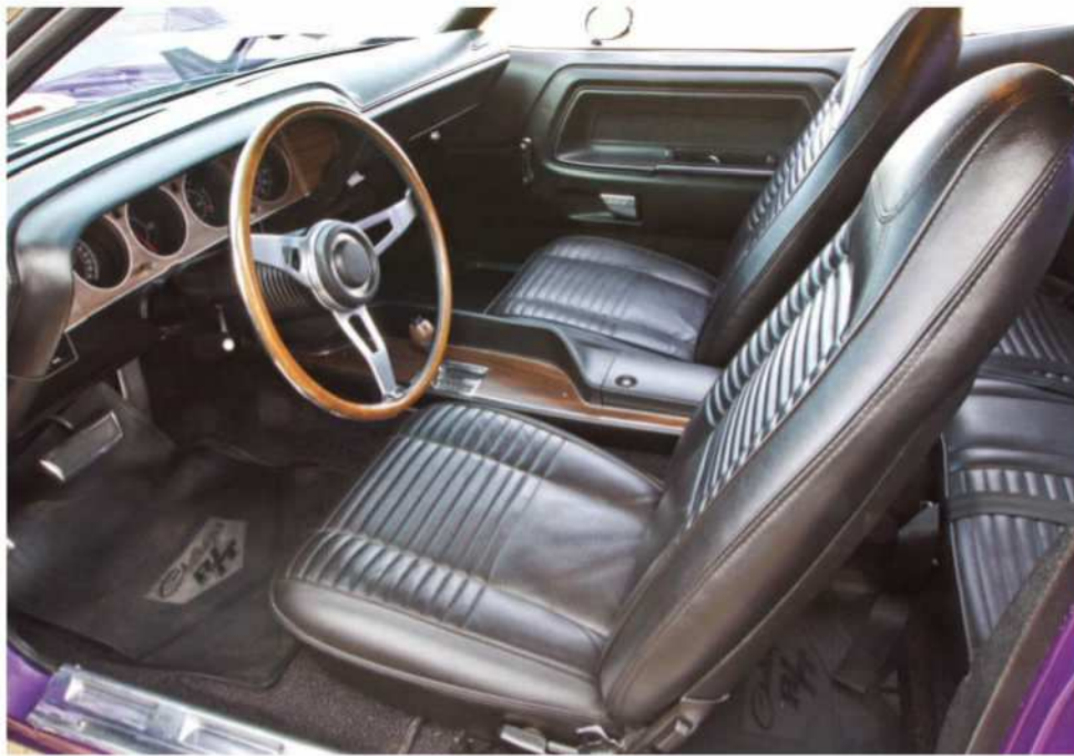
This Challenger's living quarters sported a number of options, including Rim-Blow wheel, Pedal Dress-up trim, Rallye instruments, console, and more. A set of 15-inch Rallye wheels were located to replace the car's mags.
