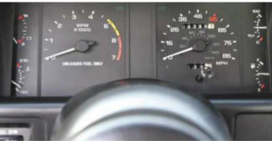
The new dash included revised instruments; V-8 cars have a 7,000-rpm tach. Speedometers changed to 140-mph calibration in '89.
