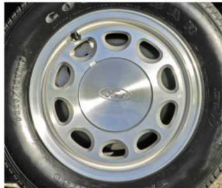
The LX 5.0 had the 15-inch "10-hole" wheels from the '85-'86 GT from '87-'90 (left); starting with the '91 model year, all 5.0 Mustangs got 16-inch "pony" wheels (right), usually in silver clearcoat.
